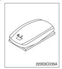
(1) When the switch is pressed ON position, the swing parking brake is locked and swing control is not available by shut off the swing pilot pressure to the swing spool.
