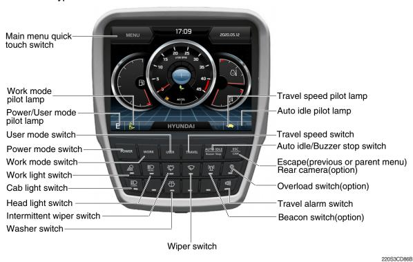
\* When some of the switches are selected, the pilot lamps are displayed on the LCD. Refer to the page 3-9 for details.
