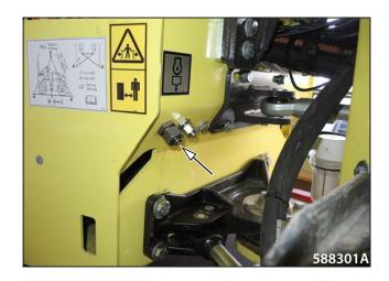
Clean the surface around the head of the oil filter. Remove the filter. Clean the seating surface for the filter gasket.
