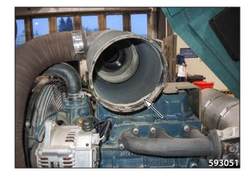
Remove the dust valve of the air filter, clean and remount.
