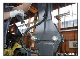
Tilt the ROPS safety frame to the back and secure it in a suitable way.
