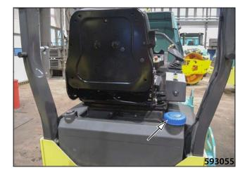
Remove the drain plug of the water tank. Rinse the tank with running water.
