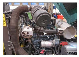
Check connections and the piping for leakage and the engine inlet opening on the bonnet for clogging (e.g. by leaves).
