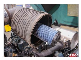
Clean the internal area of the filter and of the contact surface so that no dust is taken into the inner supply piping towards the engine.
