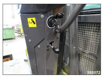
Connect the computer to the machine using a cable.
