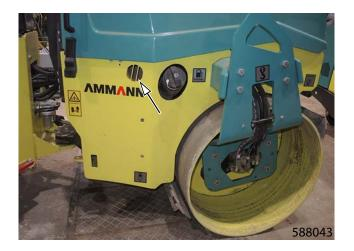
Clean the exit slit and squeeze to remove any dust trapped.
