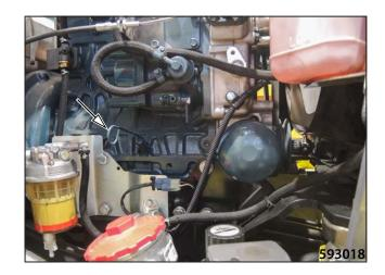
Keep the level within the range of gauge marks imprinted in the dipstick. The lower mark shows the lowest possible oil level, the upper mark indicates the highest.
