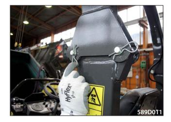
Dismount the front frame screws on the left and right sides.
