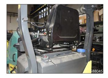
Open the tank cap and refill with clean water.
