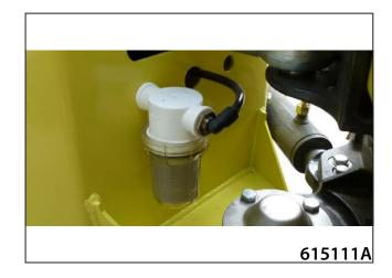
Remove and clean the sprinkler strainers.
