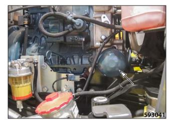
Lubricate the gasket with oil.
