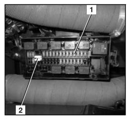
Remove the defective fuse using the fuse puller (2) and replace it.
