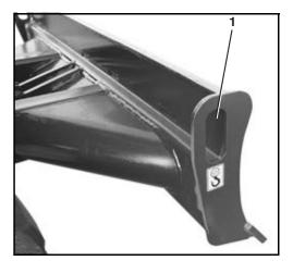
• Attach the lifting gear with shackles to the lifting eyes (1) on each side of the boom.
