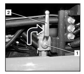
When "indirect return flow" is enabled, the return flow is directed from the implement to the return filter via the control valve and then to the hydraulic oil tank. In this case, return flow can be via the left or right auxiliary port connector (according to the position of the auxiliary port pedal) of the arm.
