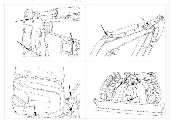
• Lubricate all greasing points with grease – see the "Recommended lubricants" section (page 118) – until fresh grease emerges.
