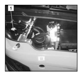
Open the central coolant drain plug (1) and drain the coolant completely.
