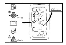
If a fault occurs in the charging system during operation, the engine must be stopped immediately. The charge indicator (1) lights up, the warning light (2) flashes red and the display message as in the figure on the right appears.
