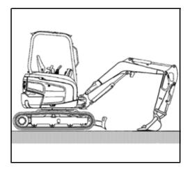
Check the oil level in the sight glass (1). The oil level should be half way up the sight glass. Carefully check the position of the hydraulic cylinders before topping up the oil. For more information see the "Topping up/changing the hydraulic oil" section (page 139).
