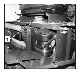
The grease gun must be stowed in the storage location (1) behind the left service cover on the swivel frame.
