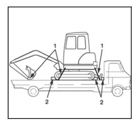
• Lock the excavator after hoisting.
