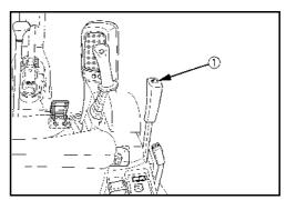
A tone sounds and the indicator (1) shines. Renewed operating of the push button travel speed switches back to normal speed. Besides, audible signal sounds and the indicator goes out.
