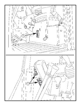
The heater valve (1) in the engine compartment regulates the supply of the heat exchanger with hot water from the cooling cycle.
