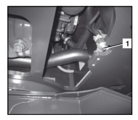
• Remove the coolant expansion reservoir (1) and drain it, cleaning it if necessary. Refit the reservoir.
