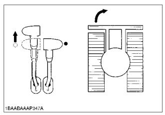
2. Pull the left drive lever backward; the excavator will turn in the direction of the arrow of the illustration below.
