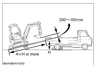
For additional safety, use blocks or supports under the ramps and the truck bed.
