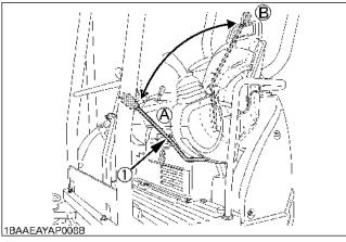
(1) Lock lever for control lever (A) "Unlock" (B) "Lock"
