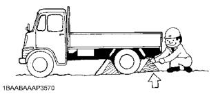
2. Use mounting brackets to secure the ramp properly. Connect the ramps directly to the truck bed.
