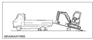
4. Align the ramps and the tracks and then drive the excavator slowly up the ramps with the dozer in the front. After ensuring that the tracks are completely on the truck bed, swivel the upper body around to the back of the truck. 5. Block the tracks and tie down the excavator with suitable chains and approved method (check appropriate state regulation).
