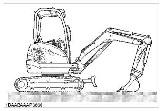
Check the oil level as to whether it lies on the center of the gauge at normal temperature (10 to 30 ℃ (50 to 80°F)).
