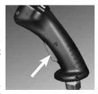
on the switch on the joystick. As soon as the switch is released, anti slip valve is released. The function of the anti slip valve depends also on the position of the drive release switch:
