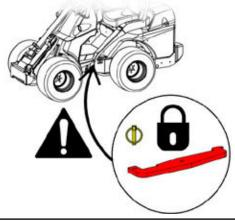
Always lock the frame lock before transporting or lifting the loader. Also remember to remove the frame lock and test the steering of the loader after transport.
